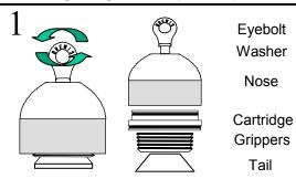
Unscrew the rear eye. Place the towing head on it's tail and unscrew the eyebolt. Lift off the nose and cartridge.
