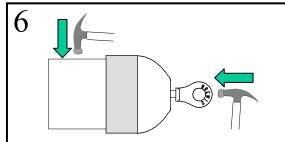
To remove the towing head unscrew the eyebolt.
