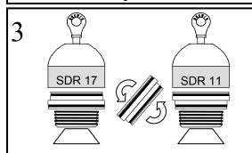
Place the cartridge back on top of the grippers with the required size downward.
