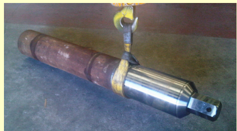
Ø219mm swivel with male hex and 1m of casing welded on
